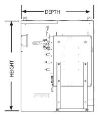
For PNI styles: height = 65" (1651mm), (up to 90") depth = 55" (1397mm).
